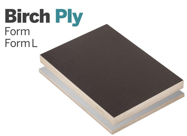
Metsä Wood Form is birch plywood, in which both sides are overlaid with phenol film and the edges are sealed. Form plywood is an ideal formwork panel for smooth surfaced concrete elements. It can also be used as a multipurpose, maintenance-free panel for various other uses. Metsä Wood Form is available in sizes standard, L, XL and KingSize.
