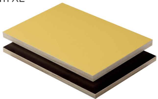
Metsä Wood Form XL is a larger size birch plywood panel with smooth phenolic overlay. Form XL is a tough-surfaced, durable shuttering panel for demanding formwork appli-cations. The durable overlays and large panel sizes ensure multiple uses and a high quality concrete finish with fewer joints. XL panels enable larger one piece components.
