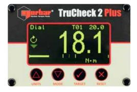
TruCheck™ 2 Plus display showing helow target tolerance
