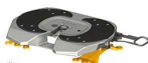
Imposed load 20,000 kg D-value 152 kN Overall heights 128, 150, 185, 225, 250 mm
